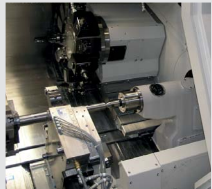
High precision, repeatable production on 7 axis CNC machines (drive shaft shown)
